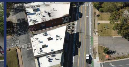
After four to three lane conversion
